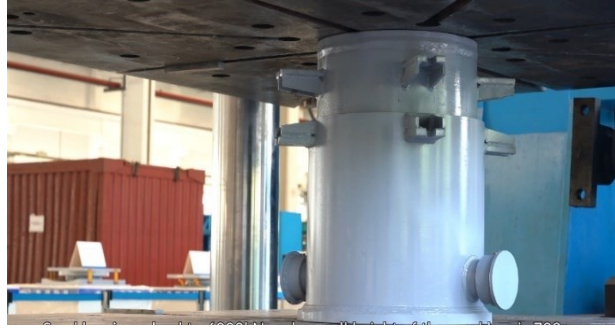
Figure 4.19 - Pre-load of the sandbox in Factory
