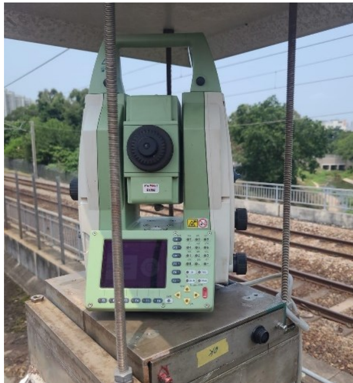
Figure 5.2 - Total Station along the railway track
